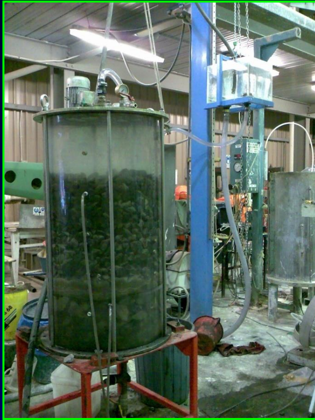
Large-scale permeability test apparatus Hydraulic Conductivity (k) of fouled ballast
